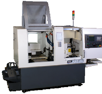
CNC Swiss Type Lathes – Bar Capacity: 13mm, 20mm, 32mm, 38mm
